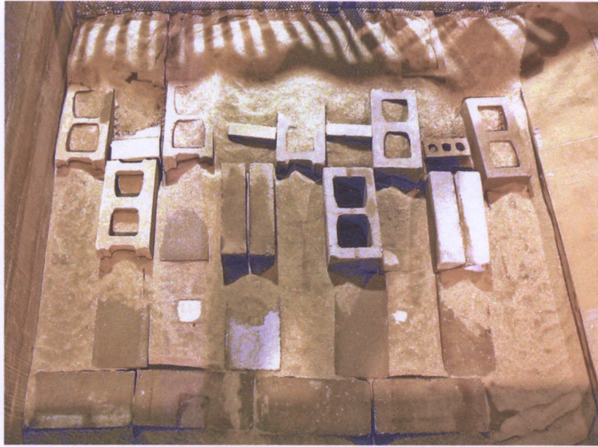
Figure 3-3 Concrete blocks arranged at entrance of channel
