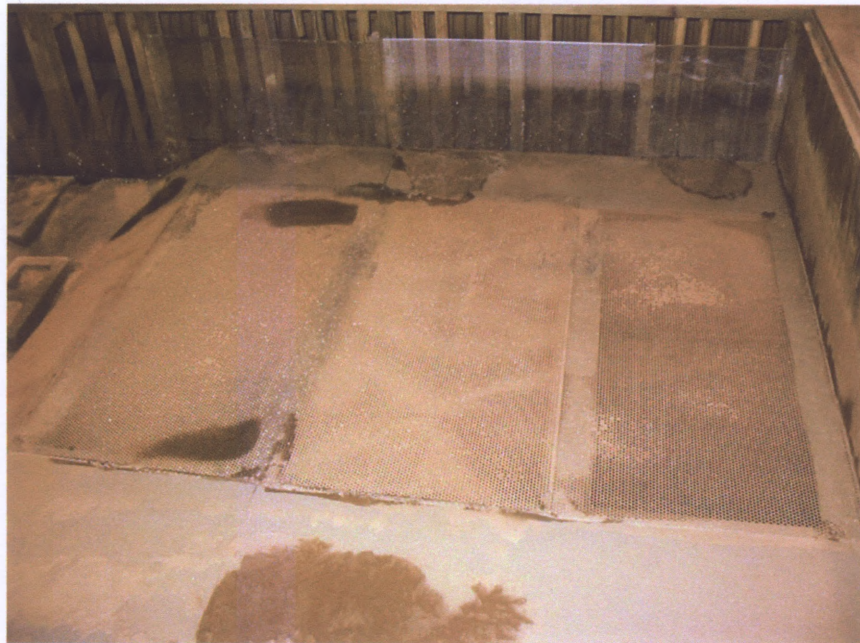
Figure 3-4 Perforated plate and sand sink at upstream end of floodplain
